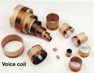
(consisting of a former, collar, and winding) of wire attached to the apex of a loudspeaker cone. Its purpose is to provide the motive force to the cone by the reaction of a magnetic field to the current passing through it. These voice coils come in different sizes range from 33.3 mm to 127.5 mm in Kraft SV,
